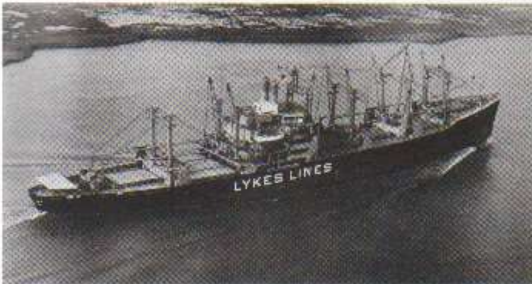
Figure 5-2. Modern break-bulk ship with capability of handling containers on deck. This Lykes Lines ship has high capacity booms. Courtesy: Lykes Bros. Steamship Co., Inc.
