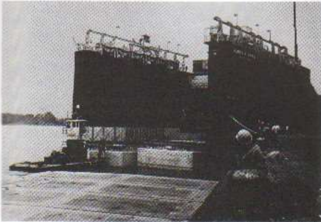
Figure 5-1. Modern cargo loading operation. Barges being loaded aboard the stern of the S.S. Almora Lykes . Courtesy: Lykes Bros. Steamship Co., Inc.
