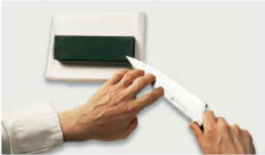
(a) Hold the knife firmly. Start with the tip of the knife against the stone as shown, and hold the edge against the stone at a 20-degree angle. Use the guiding hand to keep an even pressure on the blade.
