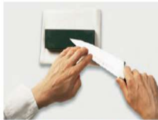
(b) Start to draw the knife over the stone. Press very gently on the blade.
