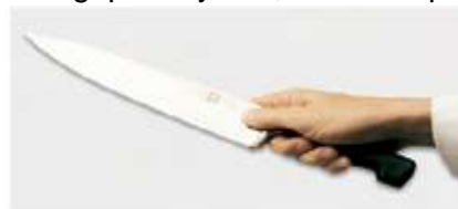
Grasping the blade of the knife between the thumb and forefinger gives the worker good control over the blade.
