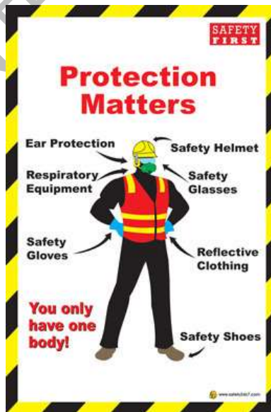
Picture above demonstrate proper use of Personal Protective Equipment (PPE)
