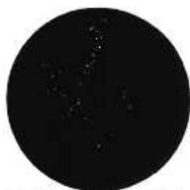
Manufactured by Crowley of Decca Radar Limited, London. Figure 2.14 - Too little brilliance.
