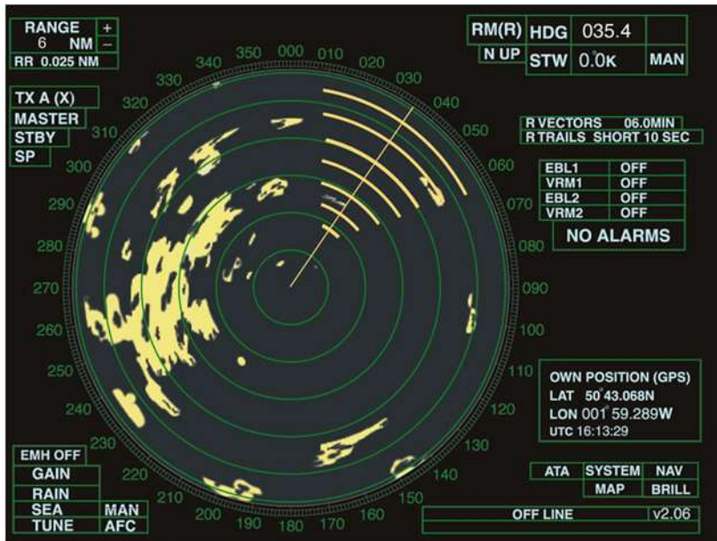
As the SART gets closer the dots turn to arcs
