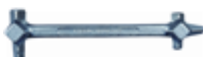
Face wrench for oil change • Universal with 10 square sizes and a screwdriver blade • Length: 220 mm • Squares male: width 8.7 / 9.5 / 10.5 / 11.5 / 13 mm • Square female: 6,8 8.7 / 10.5 to 13 / 15.2 to 18 / 16.5 to 19 mm
