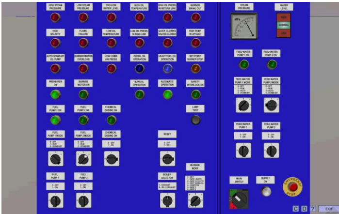
Fig. 36 Steam Boiler – control panel
