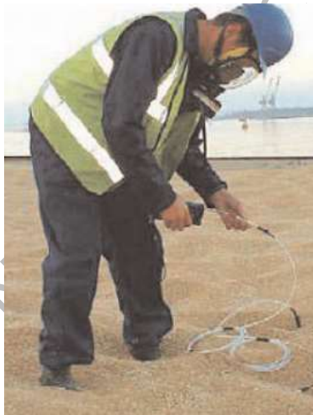
Checking the gas concentrations in the cargo prior to discharge
