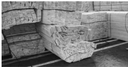
Example of poor rigidity
