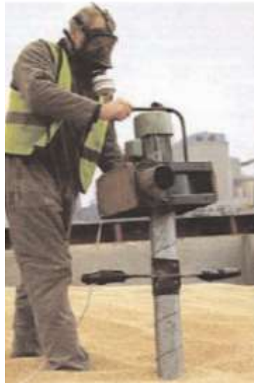
Ventilating the cargo prior to discharge
