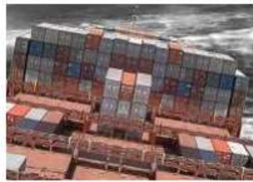
Rolling is the movement of a ship around its longitudinal axis, the rolling angle in this case being 10^{\circ} .
