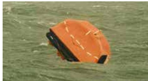
Liferaft without deployed sea anchor
