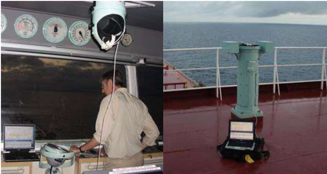
Simultaneous three axis magnetic field strength measurements in wheelhouse and binnacle
