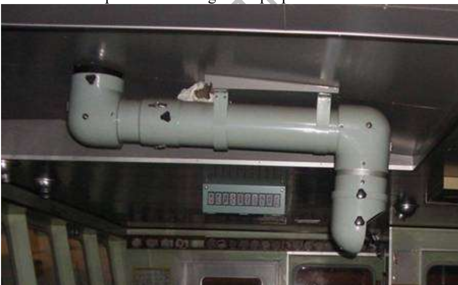
Projection assembly to view the 'standard' compass heading from the steering station.
