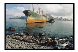
Loss of the stability: for failures in the calculations of stability or by the haste in loading the ship, or because load landslides have taken place for effects of the balances, the ship loses its capacity to correct itself after a balance. If it is not corrected, the ship ends up turning and it collapses. This is the main cause of disappearance of the ships and crews in the sea.
